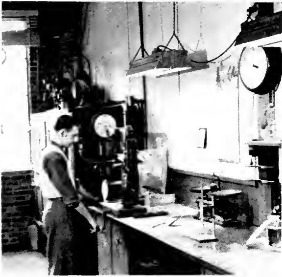
STRENGTH TESTS ARE CONDUCTED ON CEMENT, IN ADDITION TO OTHER PHYSICAL TESTS AND CHEMICAL ANALYSES
